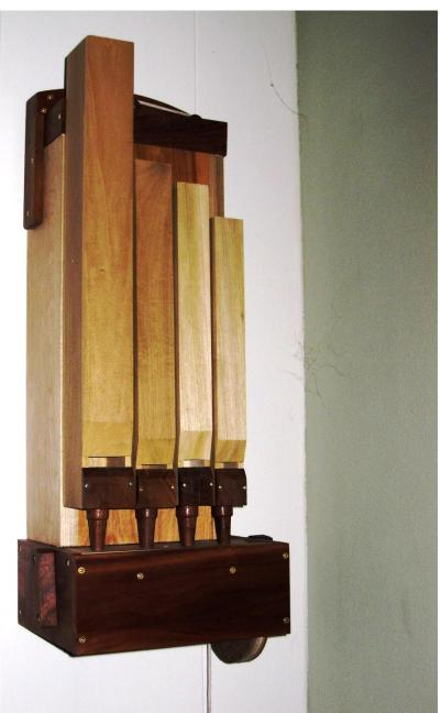
"doorgan" plays eight notes—the second half of the Westminster tune. Reset is manual (pulling the cord at the bottom), but if not reset, a transfer switch connects the original doorbell.
