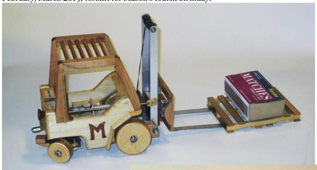
The crank at the rear moves the forks up and down. A friction brake holds the fork in position for transport. The dark knob at the right rear is a two-position fork tilt control. The lever at the lower right controls rear-wheel steering.
