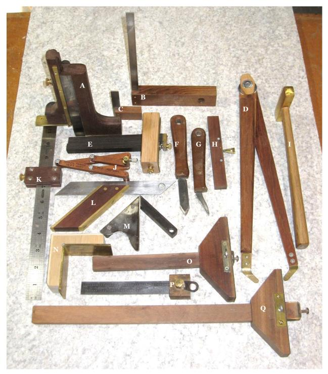
A – height gauge; B – medium try square; C – small try square; D – large inside/outside calipers; E – mortise gauge; F & G – scribing knives; H – dovetail layout tool; I – brass hammer; J – small center marker; K – clamp stop for 12-inch scale; L – miter square; M – circle center marker; N – transfer square; O – small scribing gauge; P – clamp stop for 6-inch scale; Q – large (panel) scribing gauge
