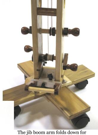
The jib boom arm folds down for shipping and storage. Note triple-pulley assembly at the top of the tower for the control cords.
