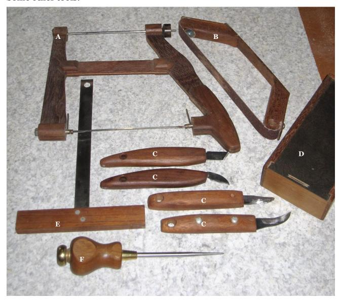
$A-coping\ saw;\ B-flex\ strip\ sander;\ C-C-C-C-carving\ knives;\ D-knife\ box;\ E-T-square;\ F-scratch\ awl,\ from\ kit\ by\ Rockler.\ I\ made\ several\ of\ these.$
