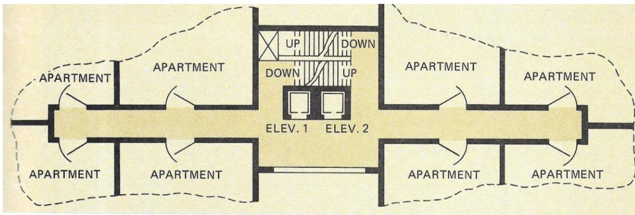
Above: hallway plan in 14-story apartment building. Note that stairs behind elevators are in a walled-off stairwell, with access doors at each level.
