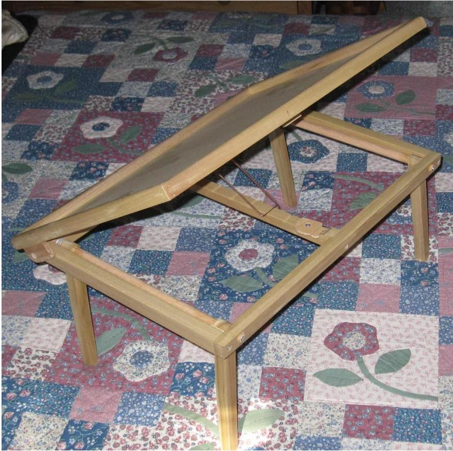
Tilting bed trays (built seven total), based on an old commercially-made tray owned by Lincoln Richards, that he found in a house he bought in NYC. The quilt was made by Grace—her original design.
