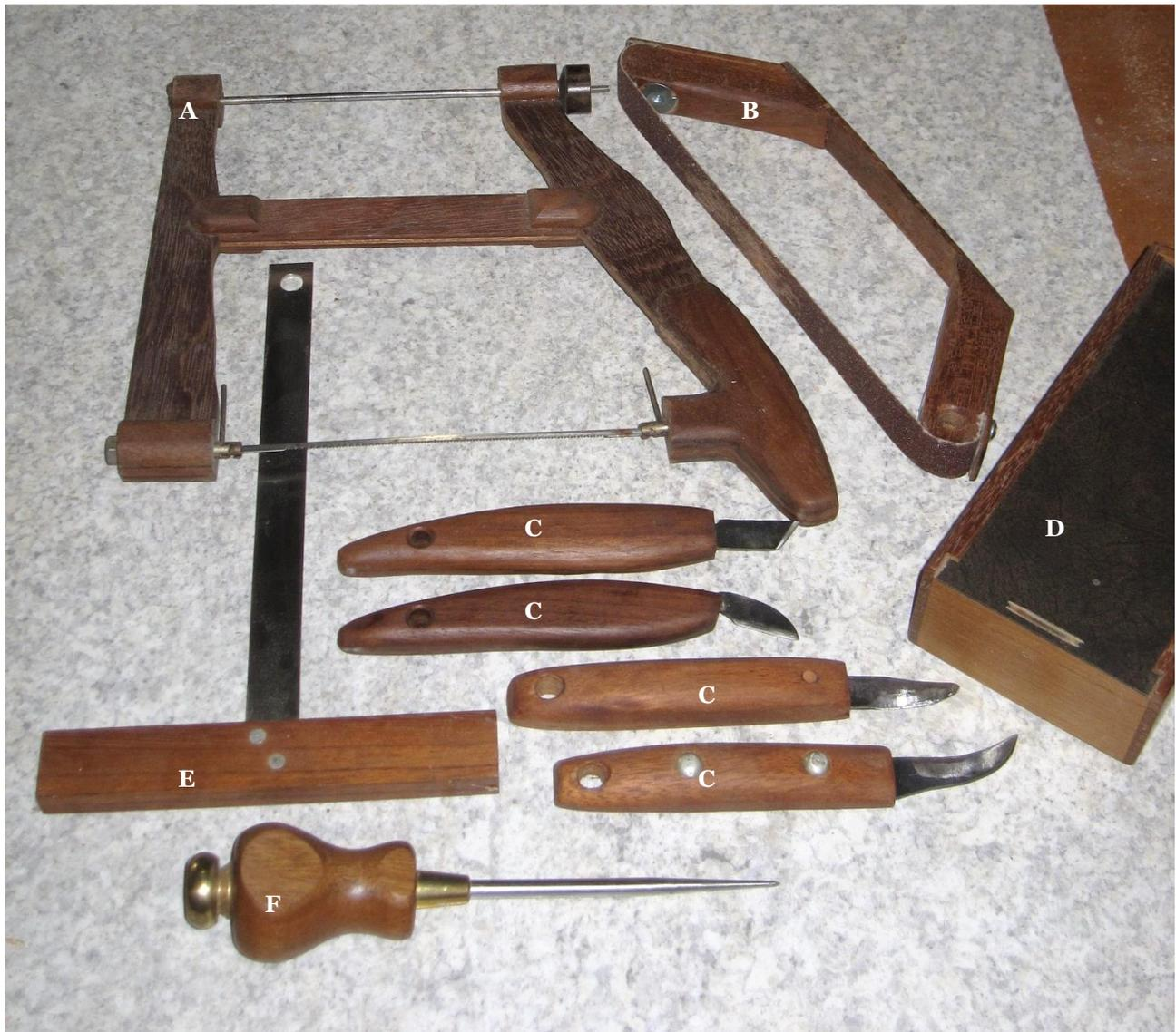
A – coping saw; B – flex strip sander; C-C-C-C – carving knives; D – knife box; E – T-square; F – scratch awl, from kit by Rockler. I made several of these.
