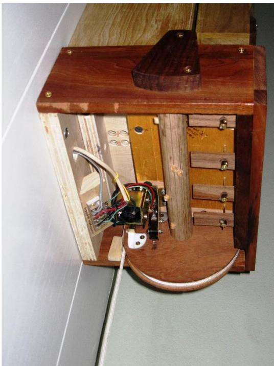
“doorgan” plays eight notes—the second half of the Westminster tune. Reset is manual (pulling the cord at the bottom), but if not reset, a transfer switch connects the original doorbell.
