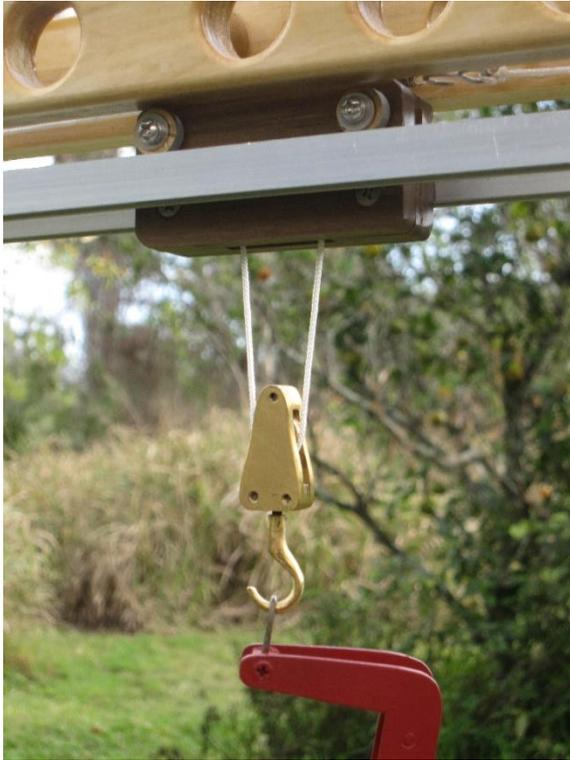
◀ I made the hook/pulley assembly from brass with stainless steel fasteners. Below—controls:
